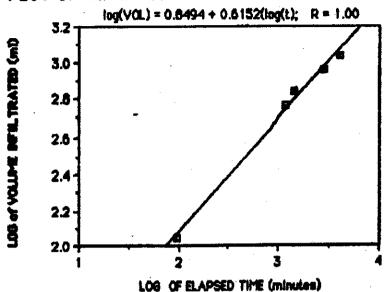
PLOT OF INFILTRATION DATA AT TANKS 1086 AND 1087
