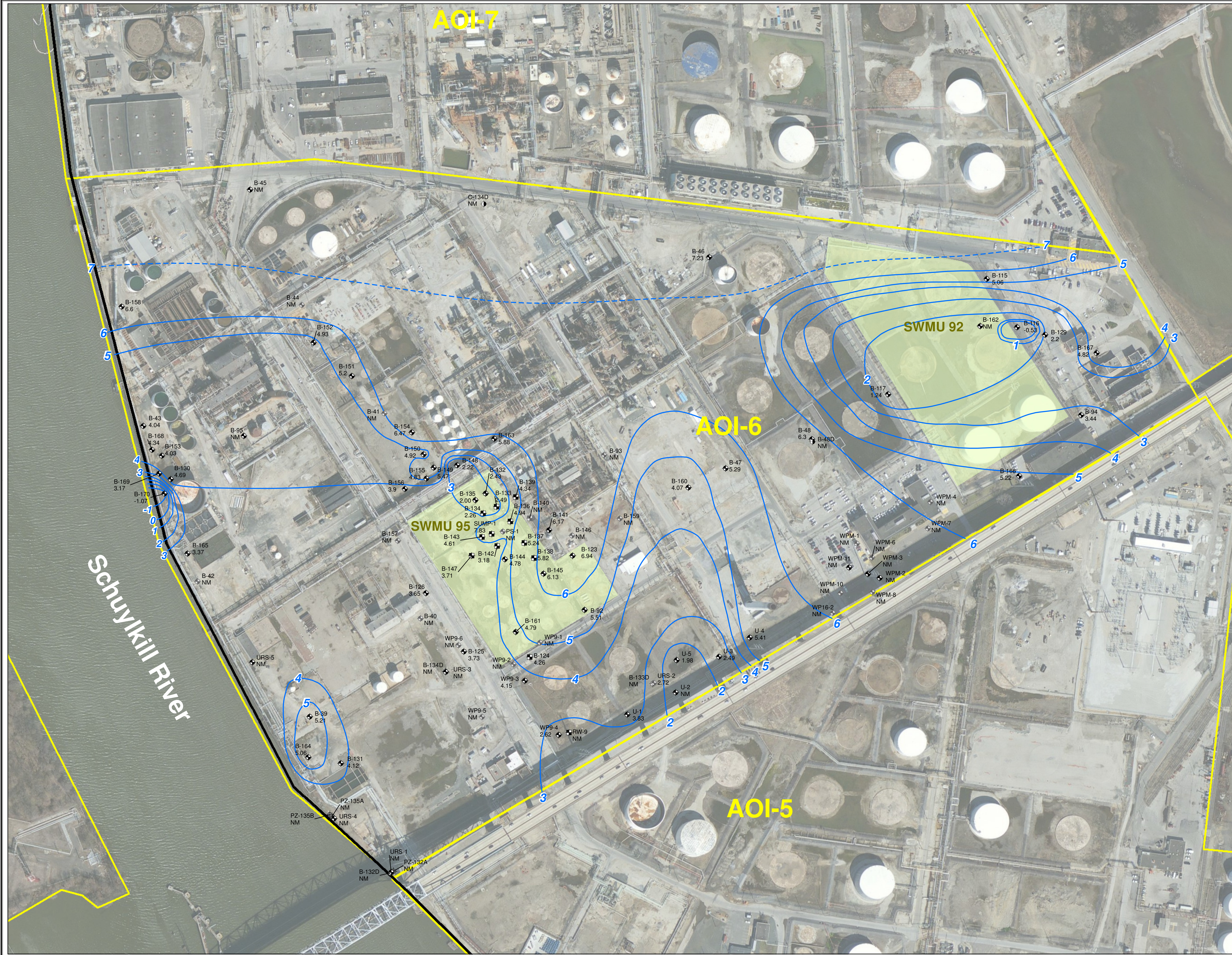
Figure 6: Fill/Alluvium Groundwater Elevations December 2012 AOI-6 Site Characterization/ Remedial Investigation Report PES Facility Philadelphia, Pennsylvania
