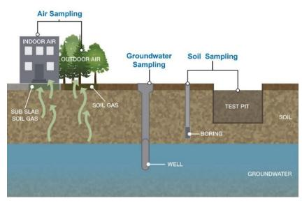
**Figure 4:** This figure illustrates some of the concepts described above. It shows 1) a monitoring well that goes below the water table for collection of groundwater samples, 2) a soil boring (installed by hand or with a drill rig) and test pit (installed by hand or with a backhoe) from which soil samples can be collected and 3) and how vapors can move upward from soil and groundwater.
