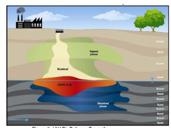
Figure 3: LNAPL Release Example (CL:AIRE, 2014)
