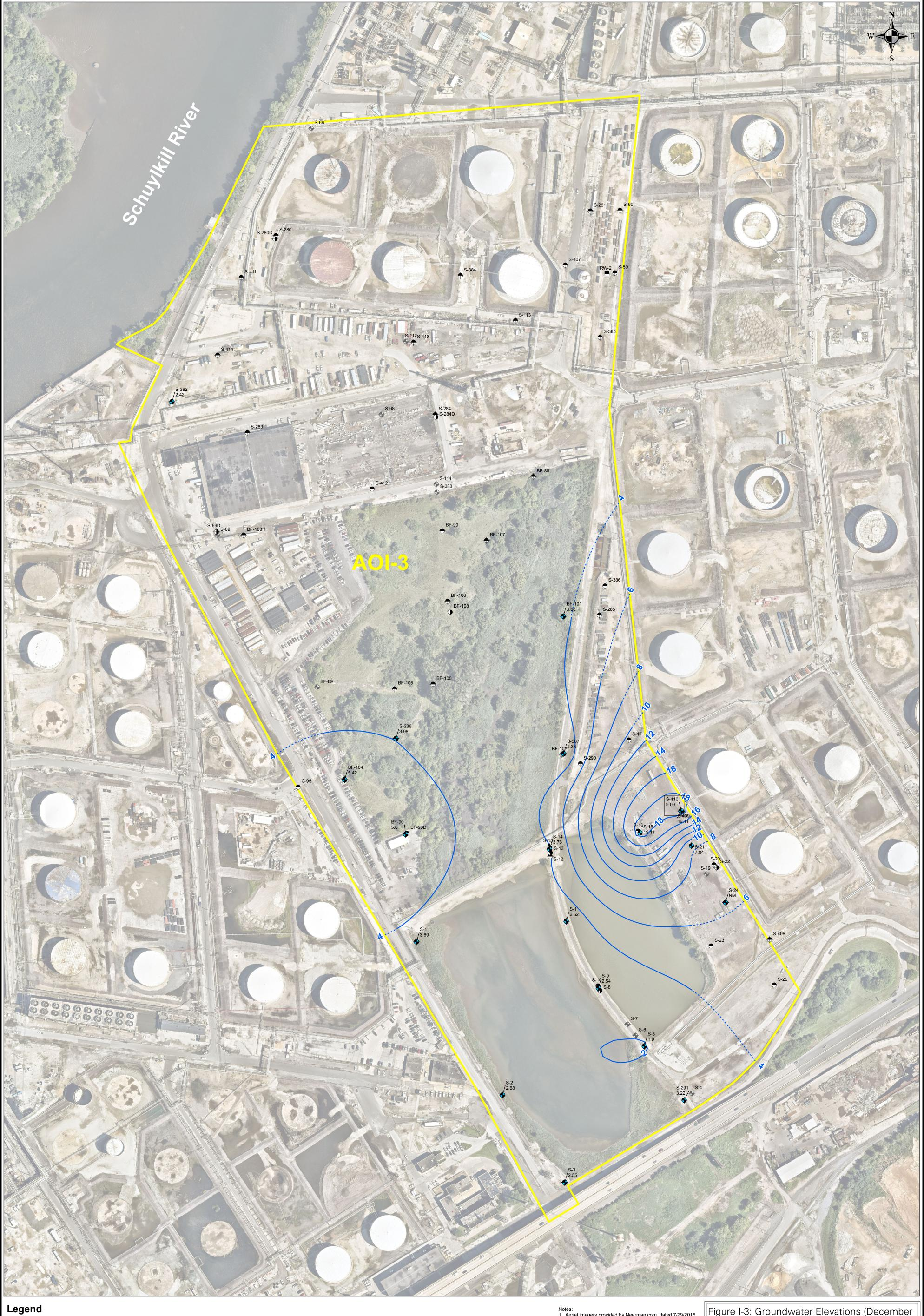
Perched Aquifer Monitoring Well and Groundwater Elevation (ft. amsl)
