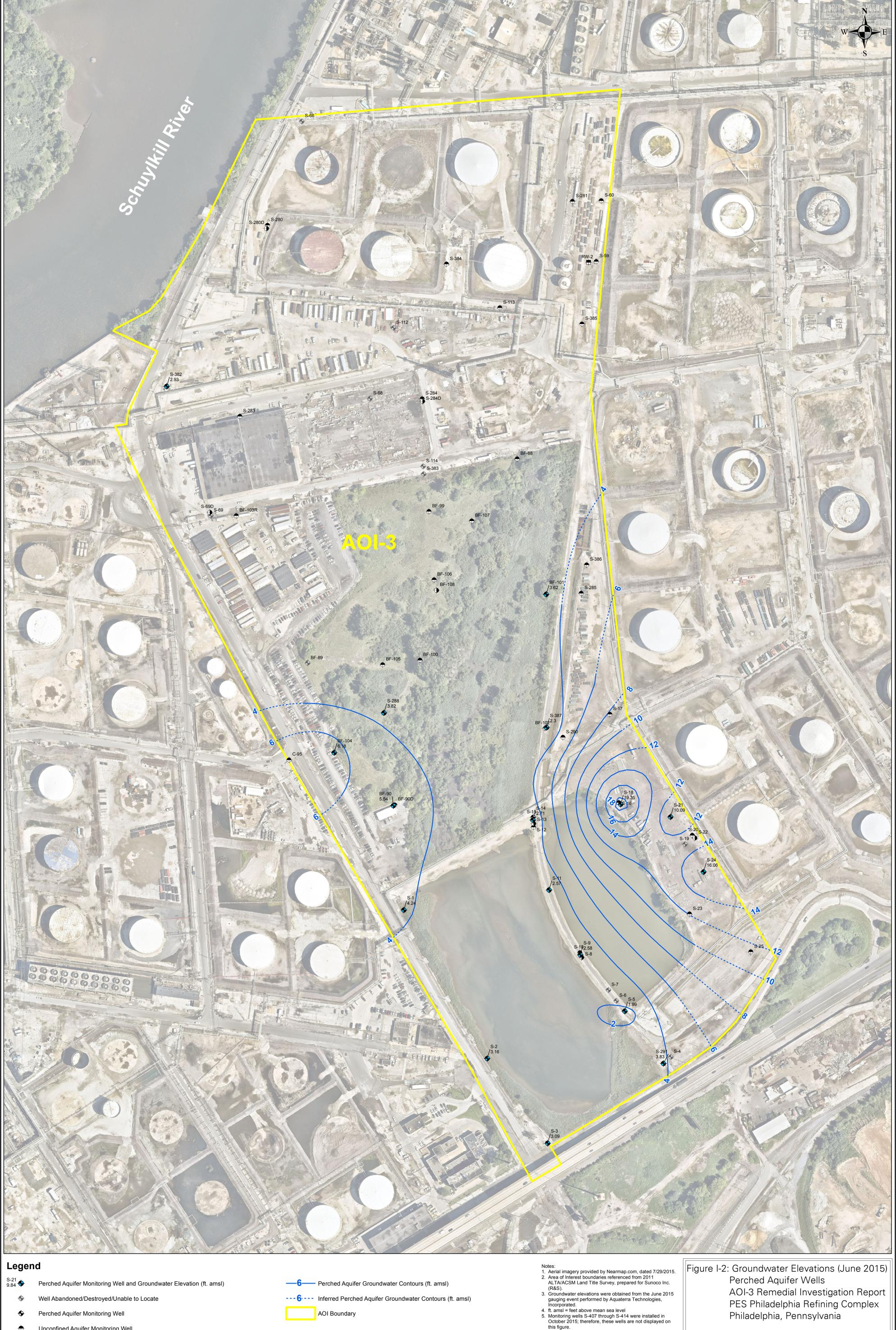
Perched Aquifer Monitoring Well and Groundwater Elevation (ft. amsl)
