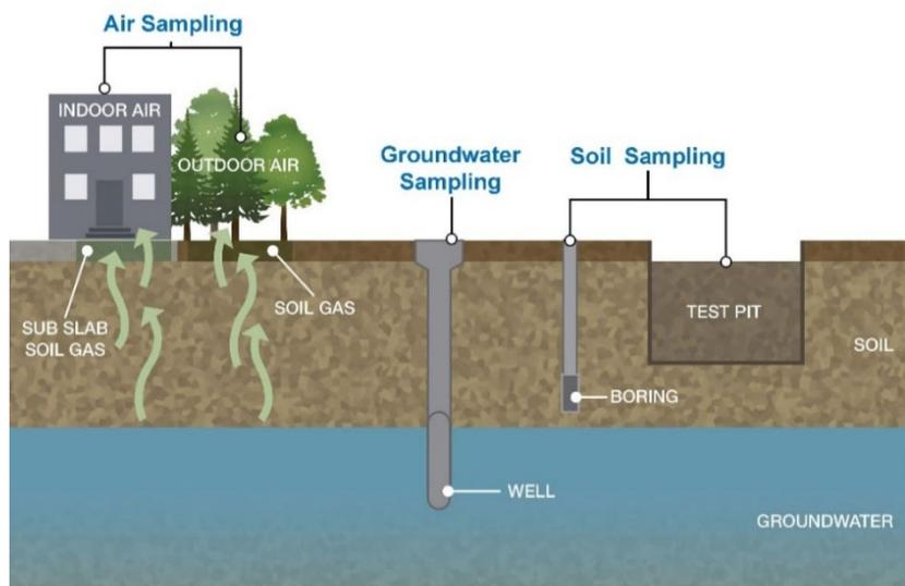
**Figure 4:** This figure illustrates some of the concepts described above. It shows 1) a monitoring well that goes below the water table for collection of groundwater samples, 2) a soil boring (installed by hand or with a drill rig) and test pit (installed by hand or with a backhoe) from which soil samples can be collected and 3) and how vapors can move upward from soil and groundwater.
